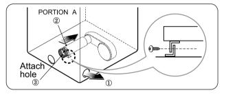
**3.** Reconnect the new duct[11 in(28cm)] to the blower housing, and Fixing the duct to the base.
