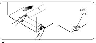
5. Insert elbow duct assembly first, through the side opening and connect the elbow to the dryer internal duct.
